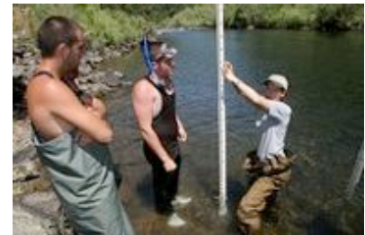
NYCP crew learn how to measure river depth with a leveling rod. (John Stumbos/UC Davis)
